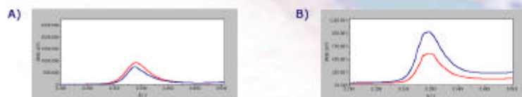
Fig. 2 Sensor response by PSA. The red lines show the peaks after ssMyc immobilization; the blue ones show the same measurements after: A) interaction with a non-complementary sequence; B) hybridization with Myc itself.
